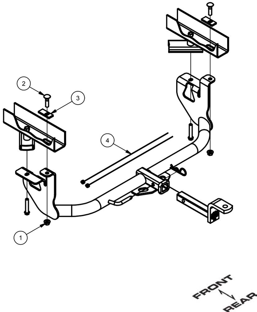
1. Remove existing M12 bolts from driver and passenger side. Retain bolts, they will be used later.
