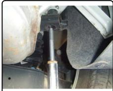
2. Reverse fishwire 1/2-13 x 2" carriage bolts and SP10 spacers through access holes in driver and passenger side frame rails.
