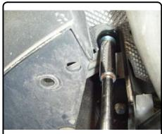
4. Hitch shown installed properly. (Re-tightened the exhaust hanger on the passenger side if loosened in Step 3.)
