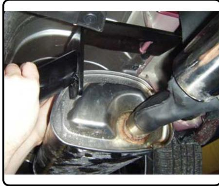
4. Loosely secure hitch with M10-1.25 x 25mm hex bolts and 3/8" conical toothed washers through existing weldnuts in outside of frame rails.
