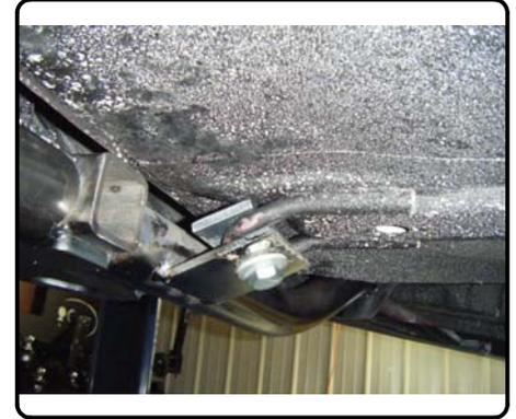
6. Torque 1/2" hardware to 75 ft-lbs and 10mm hardware to 35 ft-lbs. Raise exhaust back into position.
