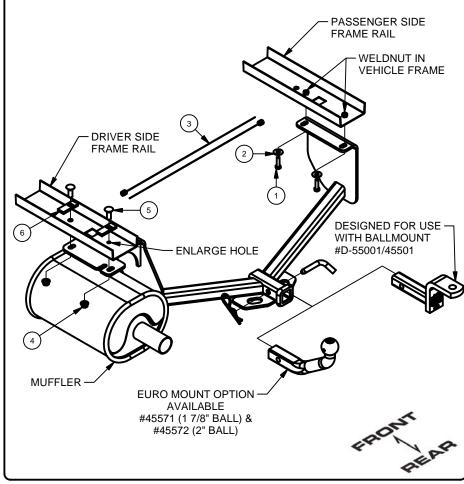
Lower exhaust by removing rubber exhaust hanger from hanger rod, two (2) places. Remove heat shield by removing four (4) hex nuts.
