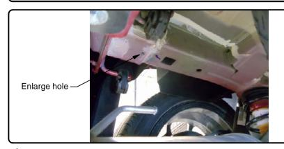
4. Raise hitch into position, taking care not to push carriage bolts back into frame and sandwiching hitch passenger side plate between frame rail and spare tire control box, if equipped. Install M8 hex bolts and 7/16" conical toothed washers into weldnuts in passenger side frame rail. Install flanged hex nuts onto carriage bolts in driver side frame rail. Torque all 7/16" fasteners to 70 lb.-ft.; Torque all M8 fasteners to 23 lb.-ft.
