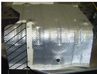
3-1/2" AREA TO TRIM HEAT SHIELD TRIMMING DIAGRAM
