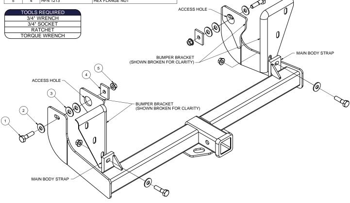
HITCH WEIGHT:  $\underline{35}$  LBS. INSTALL TIME:  $\underline{15}$  MINUTES
