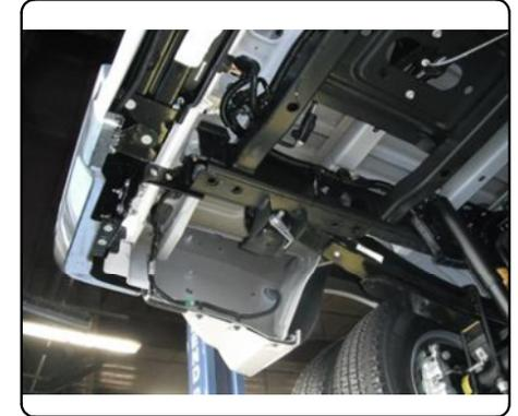
2. Place a carriage bolt and spacer into each bolt location from inside the frame rail as shown.
