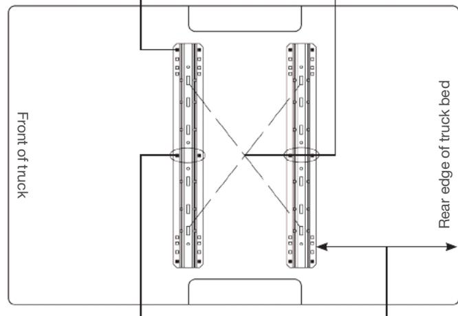
Each mounting rail must have a bolt in either of the marked holes. Check for obstructions before drilling
