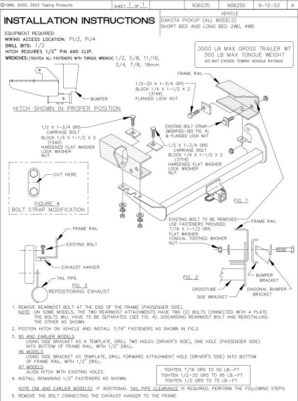
6. REPOSITION THE EXHAUST HANGER AND REINSTALL BOLT (REMOVED IN STEP 6) AS SHOWN IN FIG. 3.
