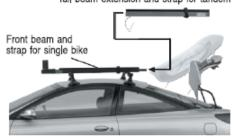
Hatchbacks or high trunk lids may require removal of tail beam to fully open hatchback Preferred carrier positioning
