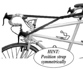
Remove and stow front wheel (Recumbents: also remove seats)
