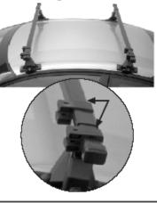
Loosen nuts to adjust rear bracket
