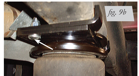
Right hand assembly (passenger side) attached with carriage bolts (R), flat washers (M) and nylon lock nuts (U). Torque to 31ft. lbs.
