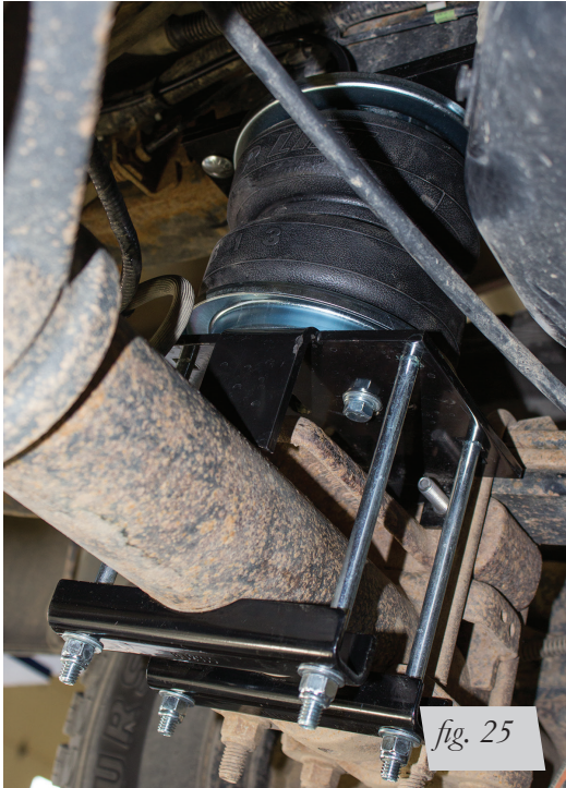
Left side (driver): front view of installation.
