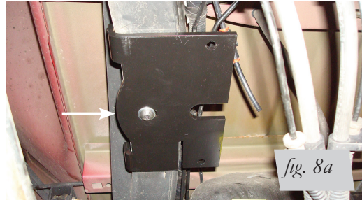
LH (driver) side. Push bracket against frame and torque to 38ft. lbs.
