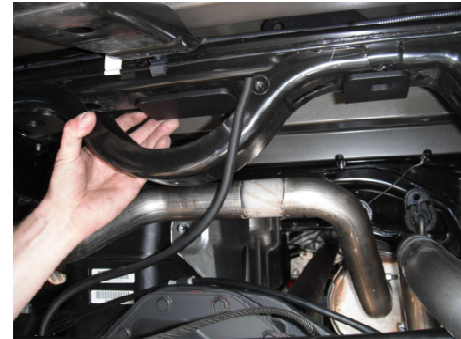
Figure 8.1: Axle Vent Hose Relocation
