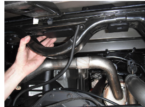
Figure 8.1: Axle Vent Hose Relocation
