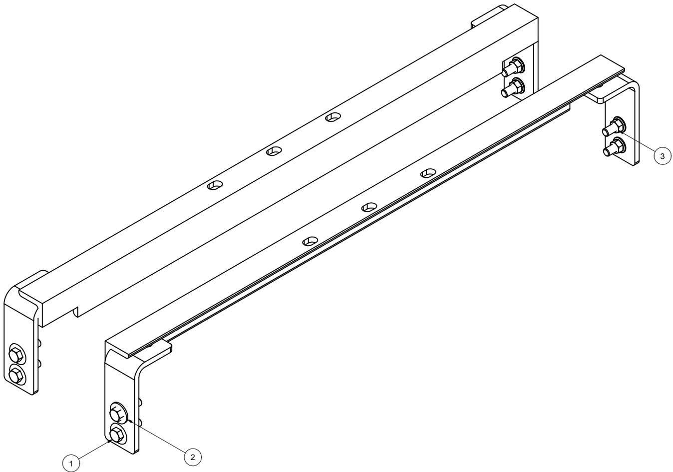
PERIODICALLY CHECK THIS MOUNTING KIT TO ENSURE THAT ALL FASTENERS ARE TIGHT AND THAT ALL STRUCTURAL COMPONENTS ARE SOUND.
