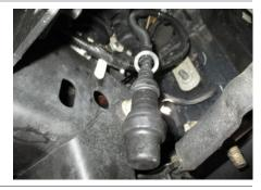
Remove the four bolts around the tow hook using an 18mm socket on both tow hooks. Pull the bumper forward and set aside for later.
