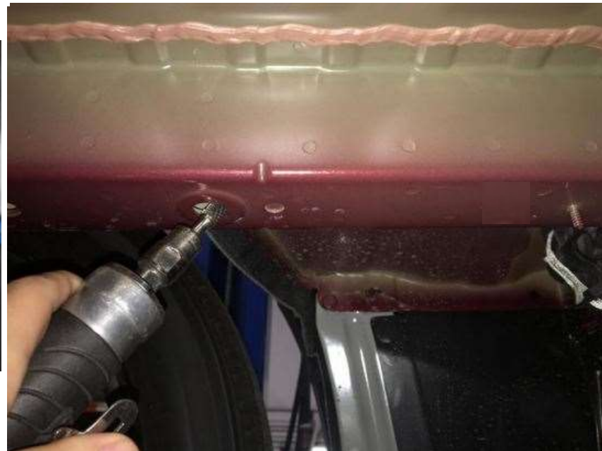
Enlarged access hole example
