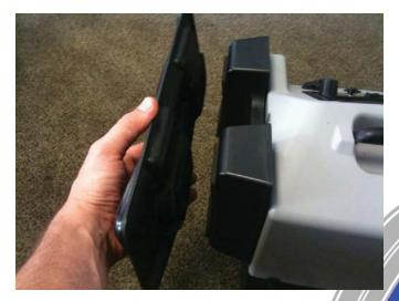
To install: Put a piece of Velcro on the brake's push pads and on the outside of the seat stiffener. The brake's push pads should line up and push against the outside of the "pockets'.
