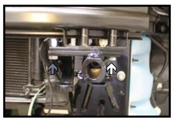
11. Reinstall the outer bumper attachment plate bolt (white). Install the 1/2" hardware on the inside edge of the plate (gray). Fully tighten all fasteners. Do this on both sides of the vehicle.
