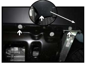
Remove the two (2) rivets from the underside corners of the fascia (inset).
