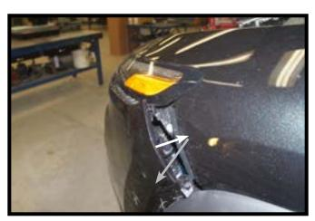
Lift the corners of the fascia up towards the fender (white) and out to release (gray).
