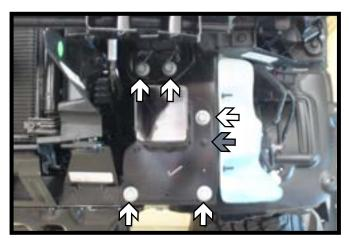
7. Using a 15MM socket, remove the three (3) bolts from the frame extension and two (2) bolts from the bottom side of the bumper (white). Using a 10MM socket, remove the nut from the fascia extension (gray). Do this on both sides of the vehicle. The extensions will not be reinstalled.
