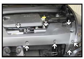
Remove the twelve (12) push pins from the top edge of the fascia cover and set aside.
