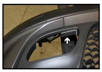
14. Trim the fascia opening as shown for clearance around the baseplate. Do this on both sides of the fascia.
