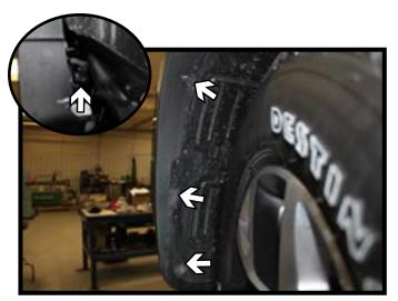
Using a 8MM socket, remove the three (3) screws from the edge of the wheel well.
