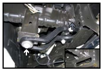
4. If equipped with tow hooks, use a 18MM socket to remove the lower bolt (white) and the two (2) upper nuts on either side of the frame (gray). Remove the tow hook and reinstall the upper nuts back onto the frame. Repeat on the other side of the vehicle.
