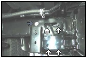
8. On the inner side of the frame, using the baseplate as a template, drill the two (2) upper frame holes and the two (2) bottom side frame holes with a 17/32" drill bit (white). Using a 1-1/4" hole saw, drill a hole in the frame above the bracket for access of the 1/2" nut wires (gray). Repeat on the other side of the vehicle.
