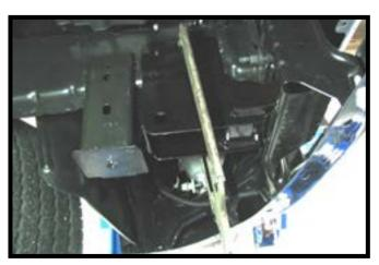
Tip the baseplate at an angle, then slide it into the opening and up to the frame. Clamp the baseplate to the frame.
