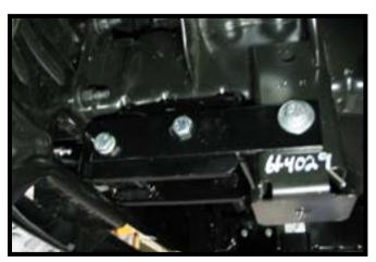
11. On the outer frame bolts, install 1/2" lock washers onto the front two (2) bolts. Then a 1/2" flat washer onto the rear hole. Fully tighten all bolts. Repeat on the other side of the vehicle.
