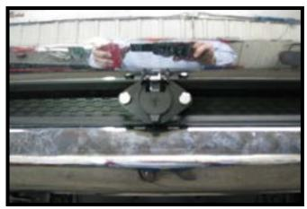
15. Center the electrical connector and mark the location of the plastic insert. Using the 1-1/4" hole saw drill a hole. Drill two (2) 5/16" holes centered with the 1-1/4" hole to mount the electrical connector. The holes on the electrical connector will need to be reamed out.
