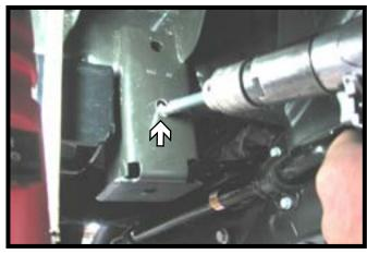
6. On the outer side of the frame, using a 17/32" drill bit, ream out the existing lower slot. Repeat on the other side of the vehicle.
