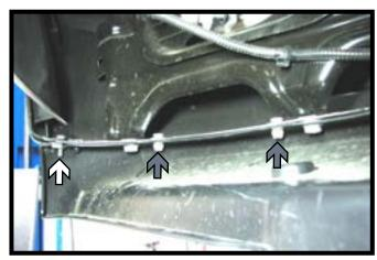
3. To remove the lower air dam, use a 10MM socket and remove the two (2) bolts in each corner of the air dam (white). Remove the thirteen (13) push pins along the seam (gray).
