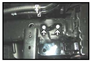
10. On the upper frame holes, insert 1/2"-13 x 1-1/2" bolts with 1/2" lock washers and 1/2" nut wires and tighten down. Repeat on the other side of the vehicle.
