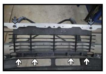
8. **2013 Models:** Using a 10MM socket, remove the two (2) screws from the top edge of the bumper (gray). Then remove the four (4) push pins from the bottom edge (white). Remove the plastic insert. Reinstall the bumper and grille to the vehicle.
