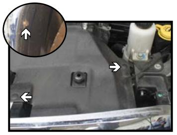
2010-13 Models: Remove the two (2) pins from the radiator cover. Do this on both sides of the vehicle. Set the cover aside.
