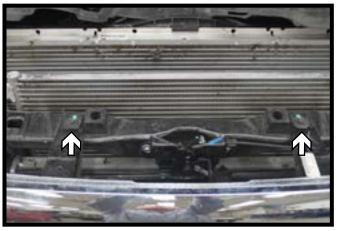
2. **2010-13 Models:** Using a 10MM socket, remove the four (4) bolts from the top of the grille. There are two (2) in the middle and one (1) in each corner. Unsnap the lower section of the grille and set aside.
