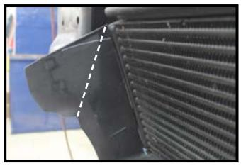
2013 Models: Trim the lower radiator shroud as shown for D-Link clearance on the baseplate. Do this on both sides of the vehicle.
