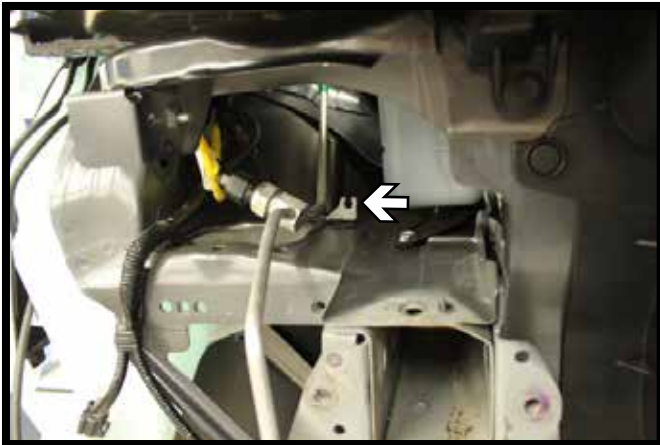
15. On the passenger side, snap the coolant line out of the bracket and carefully move over and out of the way.
