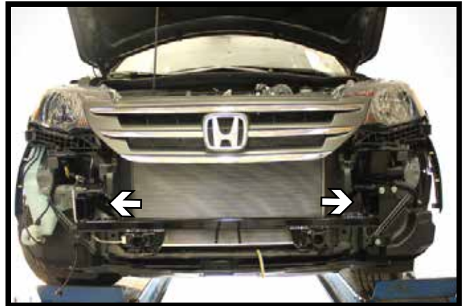
16. Slide the tubes of the baseplate into the rectangular tubing of the vehicle frame.
