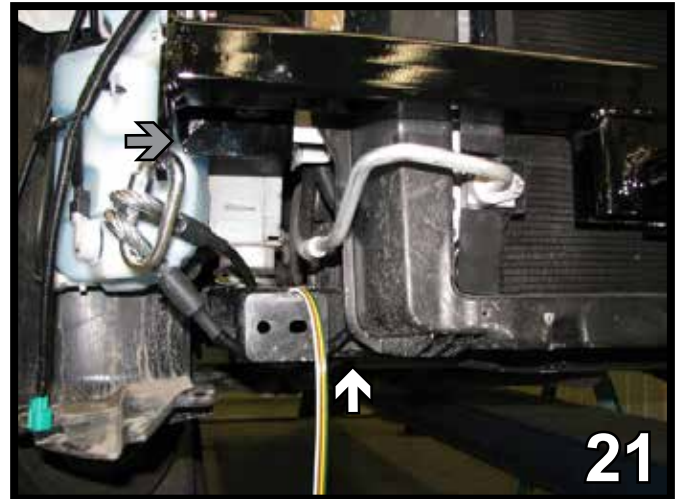
21. Attach the permanent baseplate safety cables to the provided convenience link on the baseplate (gray arrow). The photo above shows the recommended installation of the cables to frame of vehicle (white arrow). Additional options may interfere with suggested mounting; in this case secure the cables to a solid piece of the frame as described in the instructions included with the permanent baseplate safety cables. Be sure the safety cables do not rub against any hoses or moving parts. Do this to both sides of the vehicle.
