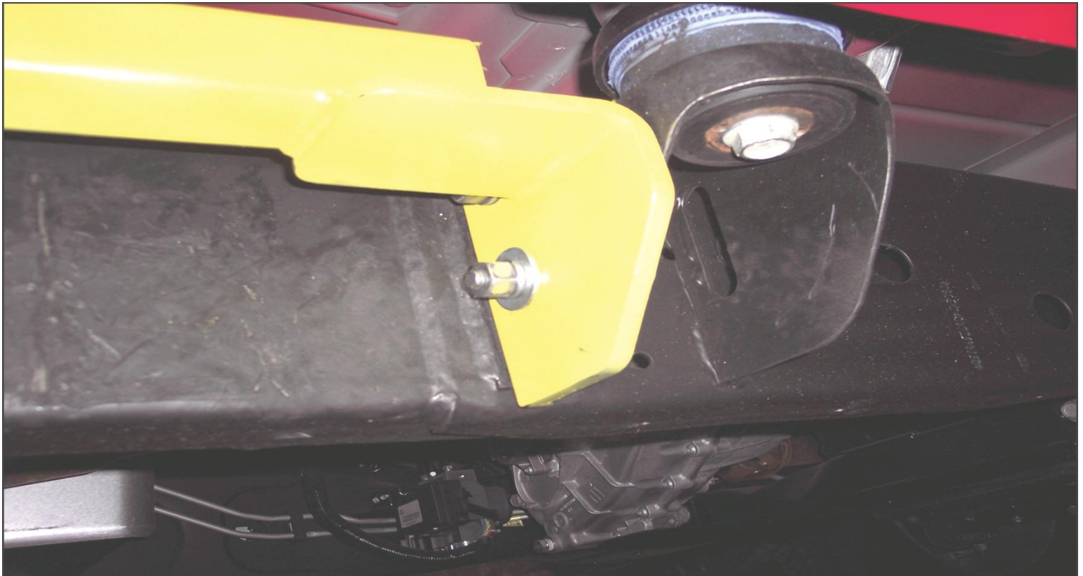
Completed Passenger Tie down
