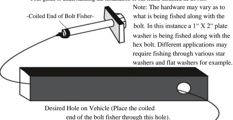
This side of the Bolt Fisher should come out of a hole where the required hardware (for example 1" X 2" plate washer) can pass through.
