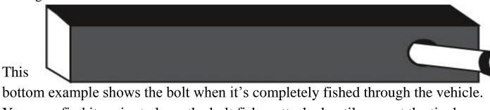
You may find it easier to keep the bolt fisher attached until you get the tie down receiver in place so that the bolt doesn't fall into the vehicle frame.
