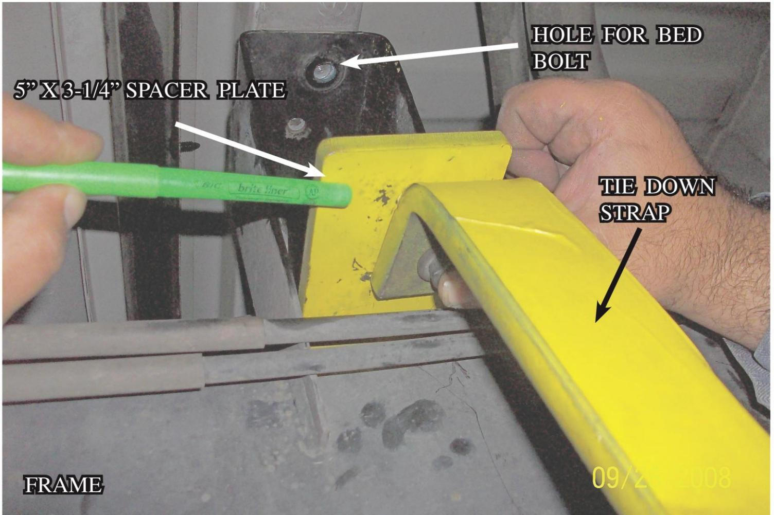
**Note:** *The spacer plate will have a hole that is offset which should face the rear of the vehicle.*
