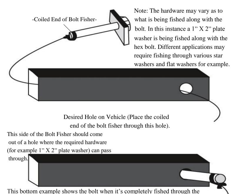
WARNING: PULLING TOO HARD ON THE BOLT FISHER CAN RESULT IN LOST FASTENERS, OR BROKEN BOLT FISHER.
