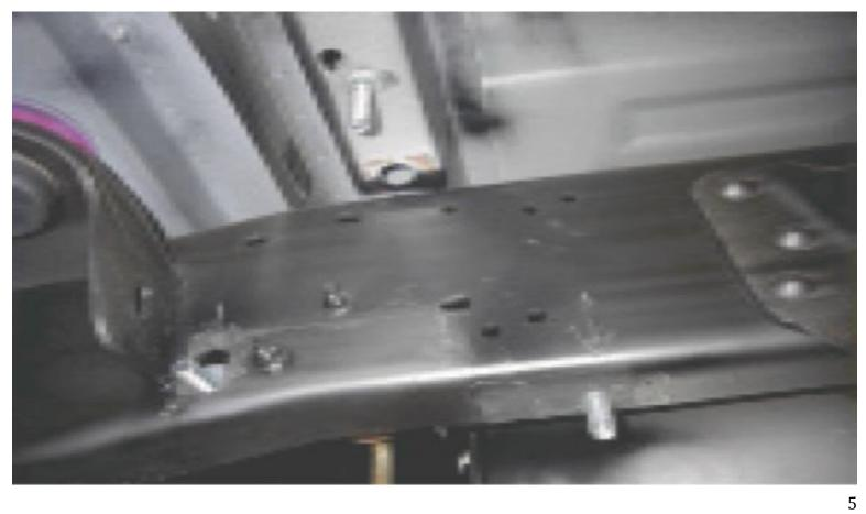
**Step 5-** Locate the support strap and two 1/2" x 3" hex bolts and two locking nuts. Choose the appropriate holes in the upper and lower channel to give at least 1" clearance between the bent insert and the lip of the bed or after market accessory.
