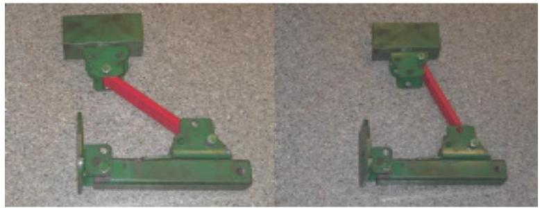
The adjustable tie downs are designed for use on trucks with running boards or steps extending onto the truck bed. When using the adjustable kit on trucks without steps or boards on the truck bed, it is very important that the support strap is **NOT** installed at a steep angle as in **photo A**. See **photo B** for approximate correct angle.
