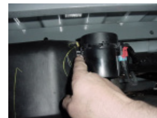
Step 2: Disengage the locking pin.
