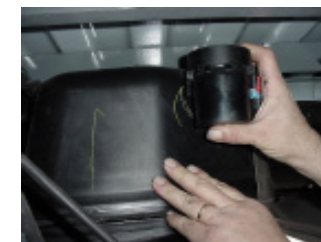
Step 3: Slide fuel valve from bracket.
