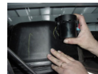
Step 3: Slide fuel valve from bracket.
