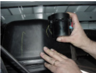
Step 3: Slide fuel valve from bracket.
