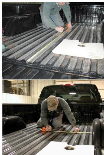
**TIP:** B&W uses a 3/4" piece of plywood as a drilling guide to prevent the hole saw from moving while drilling the 4" hole in the truck bed.
