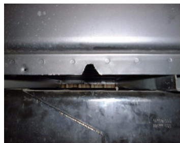
1" BED FLOOR FLANGE IN PASSENGER SIDE WHEEL WELL
