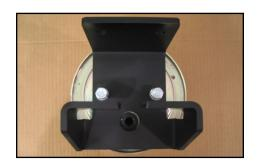
Install and tighten the 90° airline fitting in to the air spring using thread sealant.
