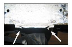
7 Install the air spring and upper bracket up onto the frame with the air port facing out towards the wheel.
