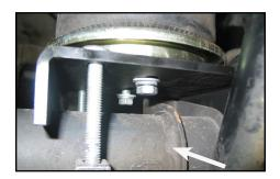
Align the air spring, by adjusting the position of it to the lower bracket slots, now snug up the bolts attaching the lower bracket to the air spring.
