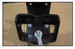
**4** Torque the upper bracket to air spring fasteners to 20 ft-lbs.
