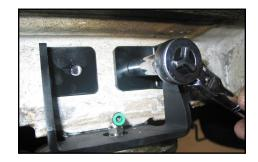
16 Torque the lower bracket to air spring bolts to 27 N•m (20 ft-lbs).
