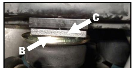
Secure the air spring assembly to the upper bracket with two  $\frac{3}{8}$ "-24 x  $\frac{7}{8}$ " hex head cap screws, two  $\frac{3}{8}$ " lock and flat washers. Make sure the upper bracket is positioned so that the bolts are screwed into the two smaller openings of the upper bracket exactly as shown. Torque to 20 ft-lbs, 34 N•m
