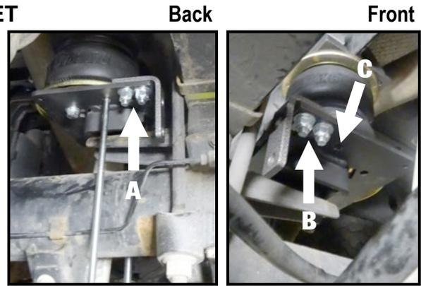
Insert a 10" carriage bolt into the unused square hole (C) from the top of the lower bracket.
