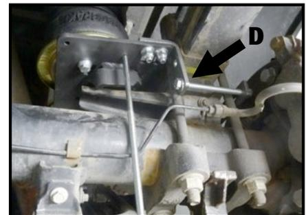
When secured to both locating brackets, the spring clamp bar will secure the lower bracket of the air spring assembly to the leaf spring, as shown (E).
