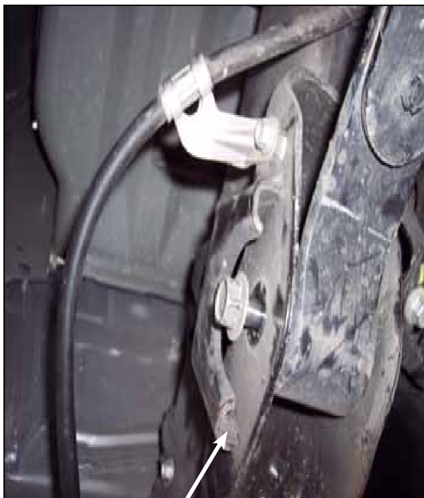
Factory bolt backed out 1/2"
