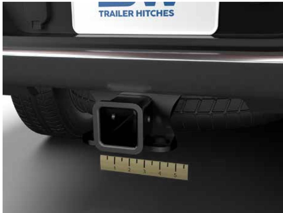
Remove any reducer sleeves (smaller tubes) from the receiver tube and measure the opening as shown. Using reducer sleeves can decrease the tow rating of your hitch and create additional noise while towing.
