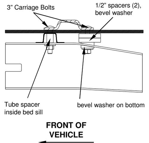
4. For the Row 4 passenger side attachment, stack two 1/2" spacers and a bevel washer, provided in the 58309 kit, to fill the gap between the bed and the frame. Use another bevel washer, conical toothed washer, and hex nut to fasten the 3" carriage bolt in place. See above drawing.
