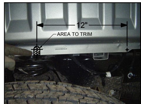
Figure 10.1: Inside Driver Side Rear Wheel Well
