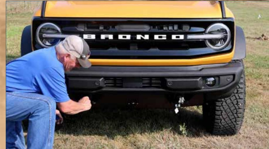
To install tabs, twist and lock. To remove, pull ring and twist.
