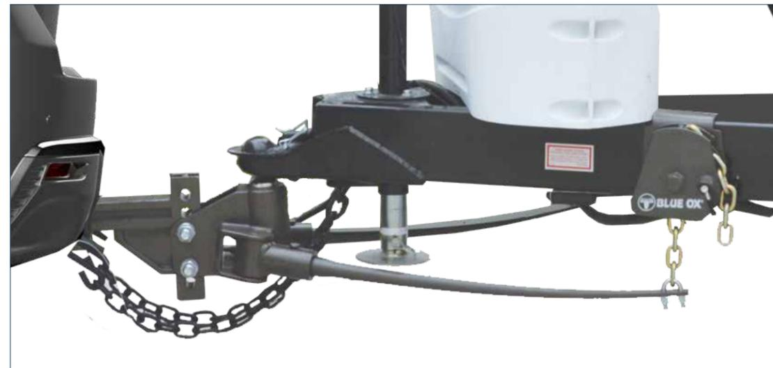
Trailers with a coupler welded underneath the frame will need to replace the standard hitch head with an underslung kit, listed below.
