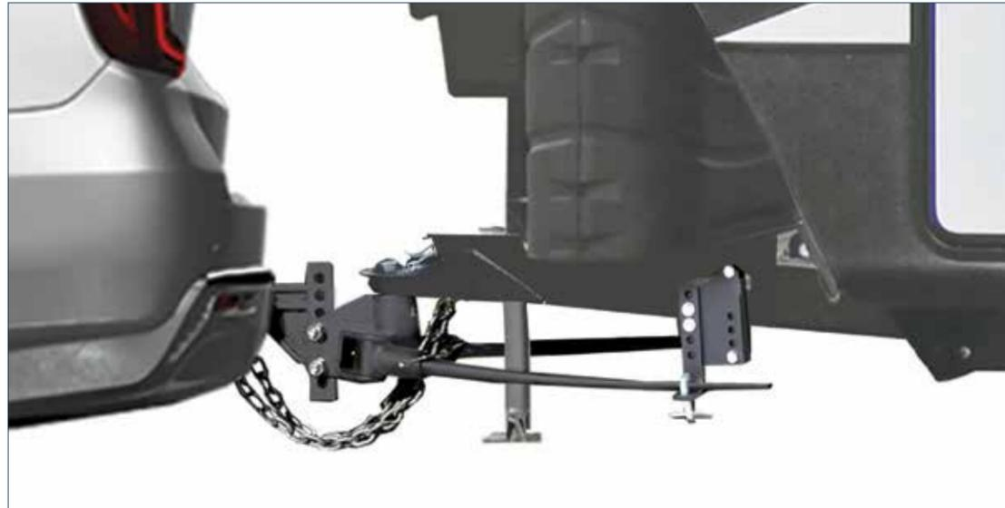
Trailers with a coupler welded underneath the frame uses the standard TrackPro Hitch Head but will need **BXW4069 Longer L-Bracket Kit**.
