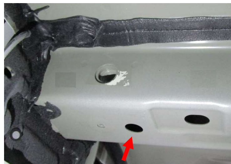
Enlarge Access Hole, both sides
